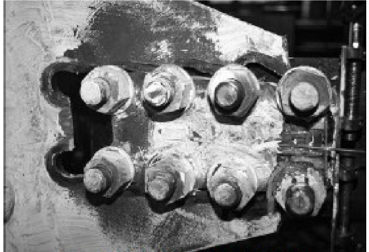
Figure 2-1. Block Shear Rupture Limit State (Photo by J.A. Swanson and R. Leon, courtesy of Georgia Institute of Technology)
