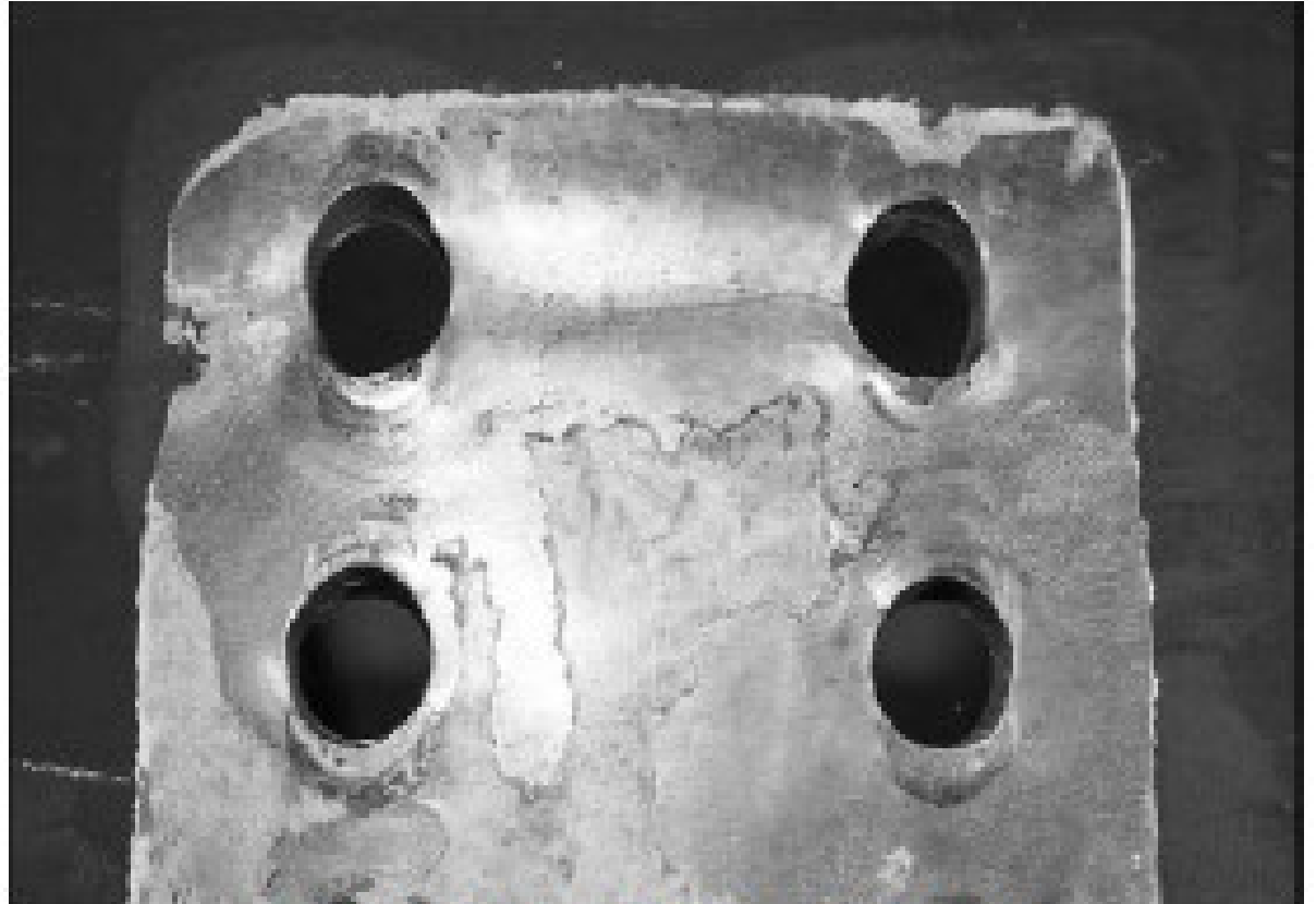
Figure 2-2. Bolt Bearing Limit State (Photo by J.A. Swanson and R. Leon, courtesy of Georgia Institute of Technology)
